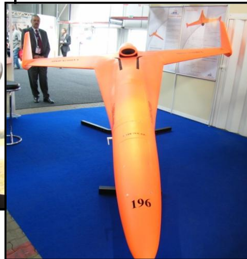
Fig. 2.4 – TJ100M installed on the wing centre section of VUT 001 Marabu
